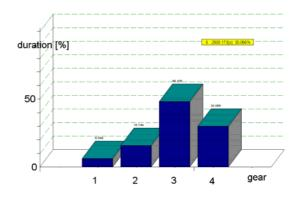
Fig.: 1: Percentage of time for gear speeds of a city bus in a city of Germany
