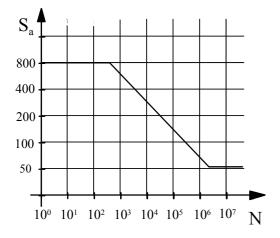
Fig. 8: S-N-curve for the critical point (notch) off the axle
