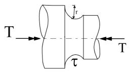
*Fig. 6: critical area of an axle under torque loading*
